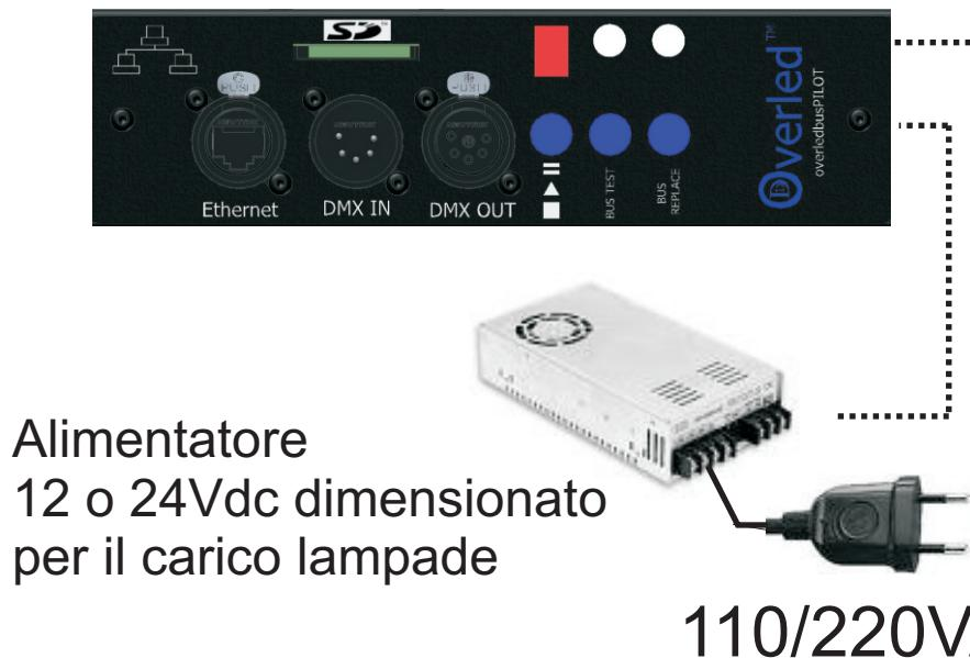
External switching power supply 12/24VDC out with correct power for the load.
