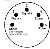
Pin 1 = signal reference = cable shield
