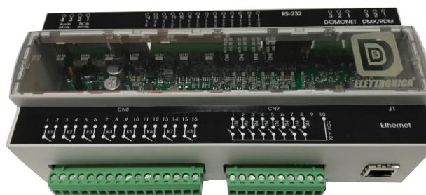
DDS920 is a ART-NET converter PLC, this device allows you to be programmed in LADDER logic, and to interact through the ART NET protocol.
