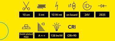
DDS835 is a 10W meter led strip with 70 led 2835 per meter. To produce our indoor flexible LED strips, we use 3-step McAdam LEDs, gold plated flexible double side PCB and constant current control inside the LED strip. Thermal conductive adhesive tape guarantees perfect heat transfer to the mounting suface. All of our product features guarantee
