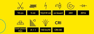
DDS763 is a 10,8W meter led strip with 70 led 2016 per meter. To produce our indoor flexible LED strips, we use 3-step McAdam LEDs, gold plated flexible double side PCB and constant current control inside the LED strip. Thermal conductive adhesive tape guarantees perfect heat transfer to the mounting suface. All of our product features guarantee
