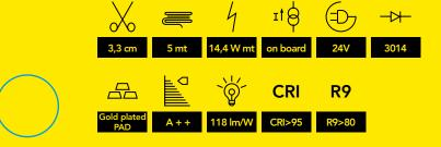
DDS535 is a 14W meter led strip with 210 led 3014 per meter. To produce our indoor flexible LED strips, we use 3-step McAdam LEDs whit high CRI and high R9, gold plated flexible double side PCB and constant current control inside the LED strip. Thermal conductive adhesive tape guarantees perfect heat transfer to the mounting suface.
