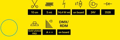
DDS532-DMX is a 14,4 W meter led strip with 50 led RGB 3528 per meter and DMX/RDM controller embedded. To produce our indoor flexible LED strips, we use high quality RGB LEDs, gold plated flexible double side PCB and constant current control inside the LED strip. Thermal conductive adhesive tape guarantees perfect heat transfer to the mounting suface.
