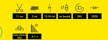
DDS737 is a 14,4 W meter led strip with 54 led RGB 3528 per meter. DDS737 can be controlled with three wires (two power and one signal). Strip control is done in indipendent section through serial signal, we suggest to use our DDS874 to control this led strip. To produce our indoor flexible LED strips, we use high quality RGB LEDs, gold plated flexible double side PCB
