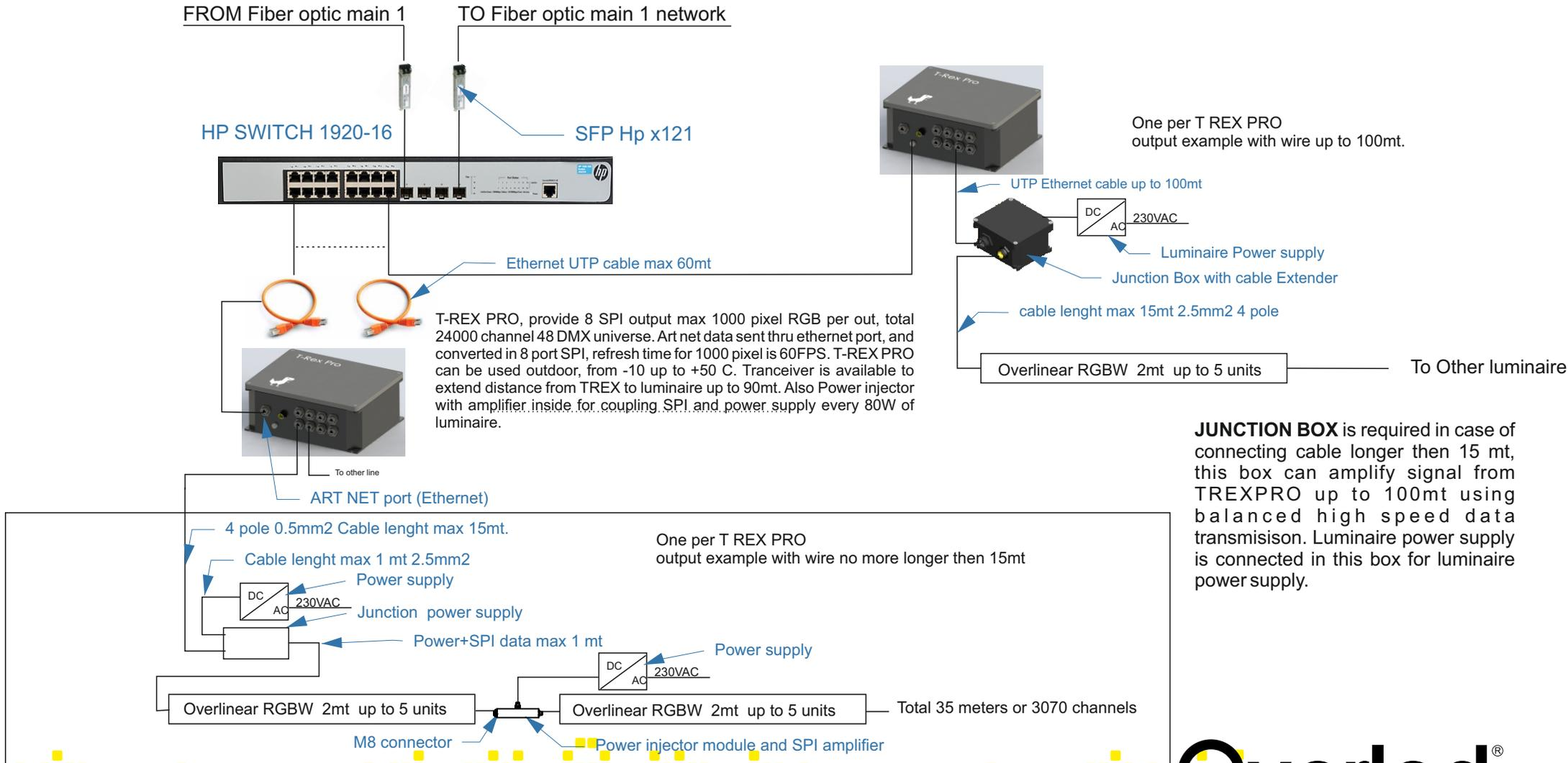
**JUNCTION BOX** is required in case of connecting cable longer then 15 mt, this box can amplify signal from TREXPRO up to 100mt using balanced high speed data transmission. Luminaire power supply is connected in this box for luminaire power supply.
