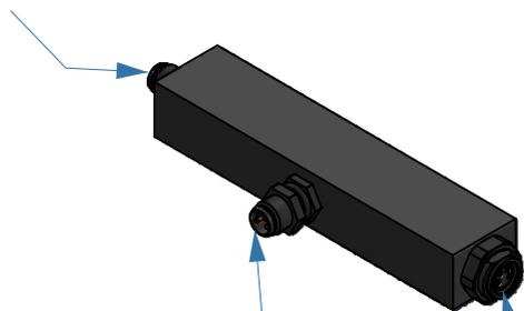
Input Data signal from luminaire
