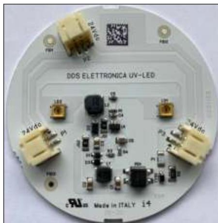
Lamp 1105, is a UVC 275nm led OEM module, developed on a metalcore pcb, with current control for the LED on board and is powered at 24vdc 2W. The light sources are dissipated directly on the PCB in metal core. There are 3 connectors with a looping connection to each other to power other modules you do not need to respect the polarity thanks to a diode bridge on board, they can be connected up to a maximum of 5 additional modules.
