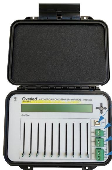
USB interface and battery charge
