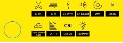
DDS1024 is a 32W meter White led strip with 175 led 2835 per meter. To produce our indoor flexible LED strips, we use 3-step McAdam high quality LEDs, gold plated flexible double side PCB and constant current control inside the LED strip. Thermal conductive adhesive tape guarantees perfect heat transfer to the mounting suface.
