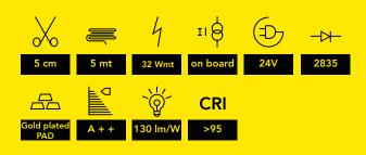
DDS1024 is a 32W meter White led strip with 175 led 2835 per meter. To produce our indoor flexible LED strips, we use 3-step McAdam high quality LEDs, gold plated flexible double side PCB and constant current control inside the LED strip. Thermal conductive adhesive tape guarantees perfect heat transfer to the mounting surface. All of our product features guarantee extra long lifetime
